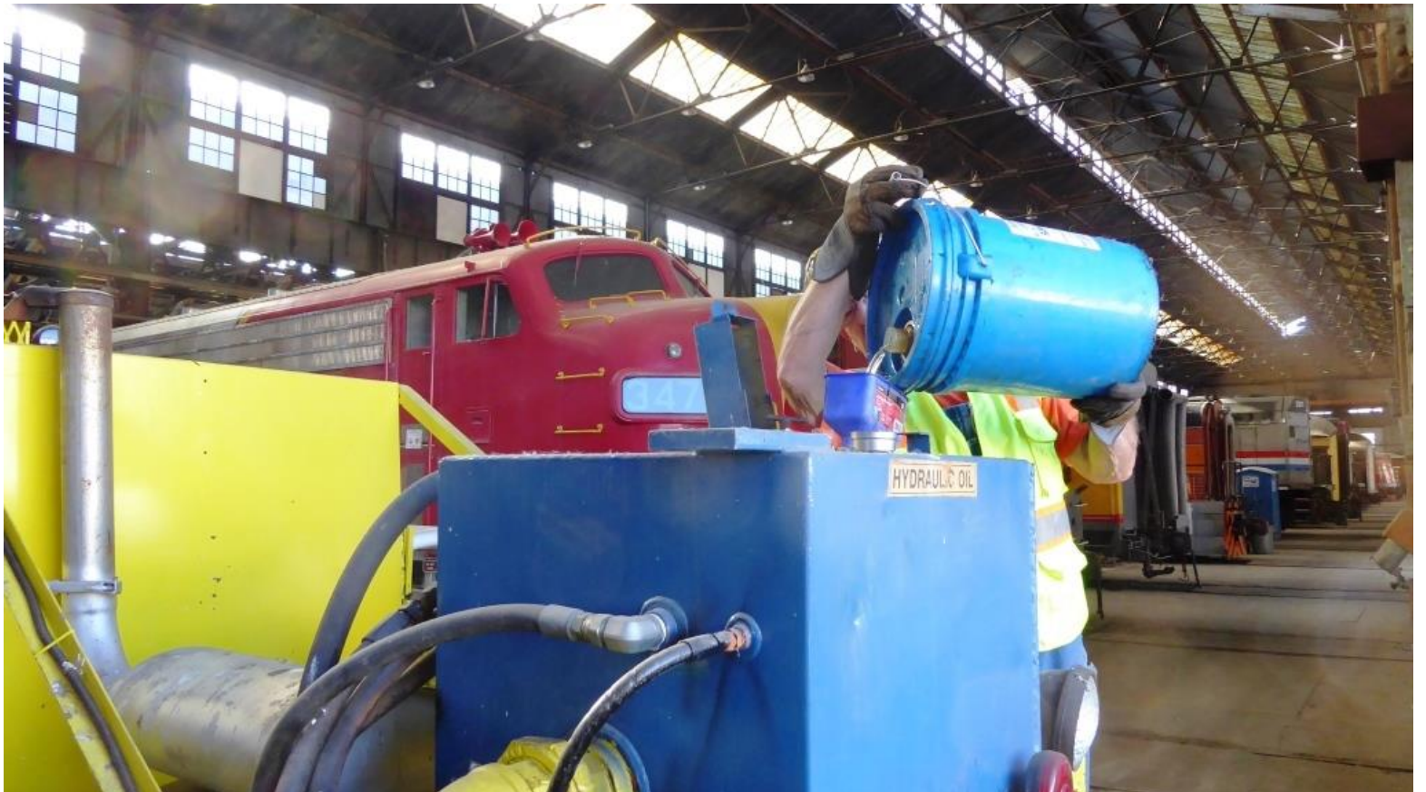
Clem adds hydraulic fluid to the spiker's hydraulic tank
