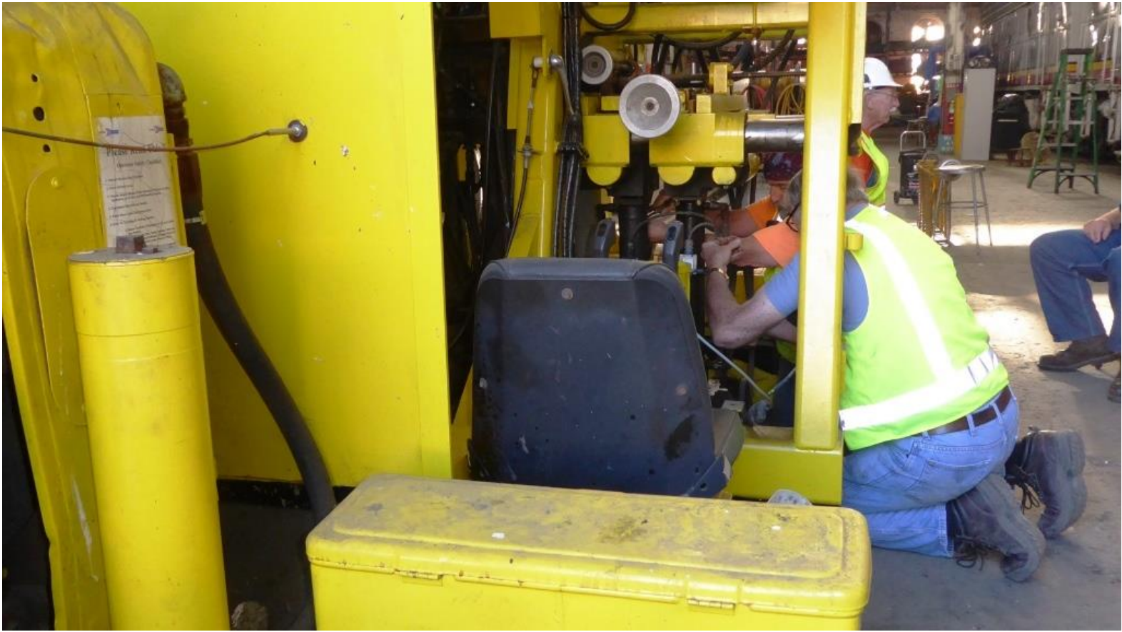
Joe and Alan make an adjustment to one of the spiking rams on the spiker
