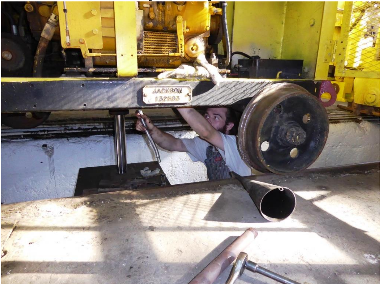
Matt, under the Jackson 125 tie-exchanger, changes the oil
